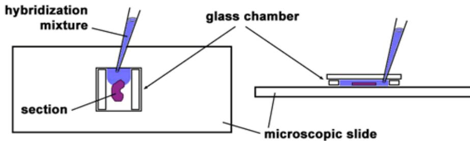
**Figure 8:** Glass-chamber for hybridization
